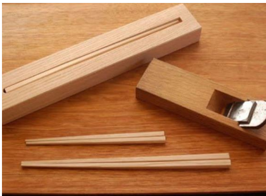
Making chopsticks with timber offcuts
